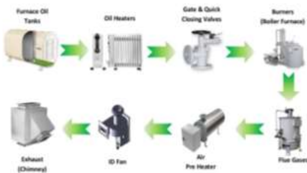
Fig. 3 Fuel oil cycle.
