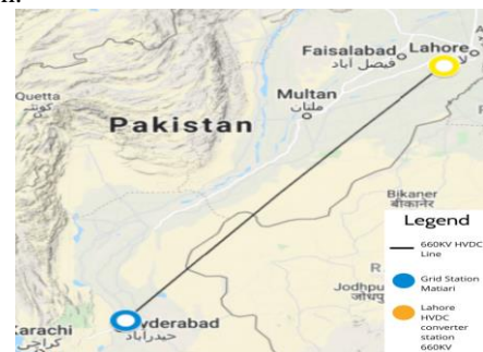
Figure 5: 660KV HVDC Line map [5]
