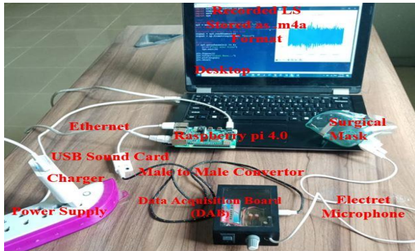
Fig. 14 Embedded System for Detection of Asthmatic Diseases.
