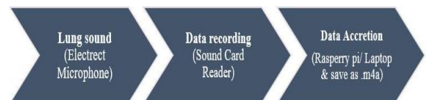
Fig. 3 Data Acquisition process for lung sounds.
