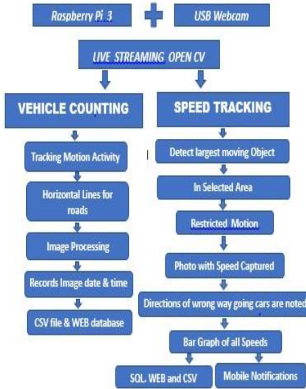
Fig 1. Procedure of the traffic controlling system using Raspberry Pi
