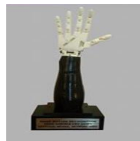
Fig. 4 3D-printed Prosthetic Hand
