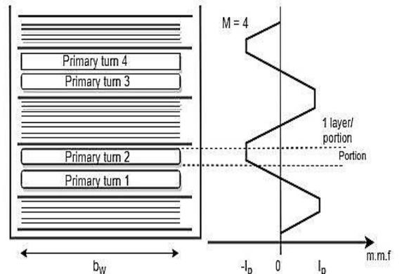
Fig. 6 Conventional double interleaving transformer winding technique
