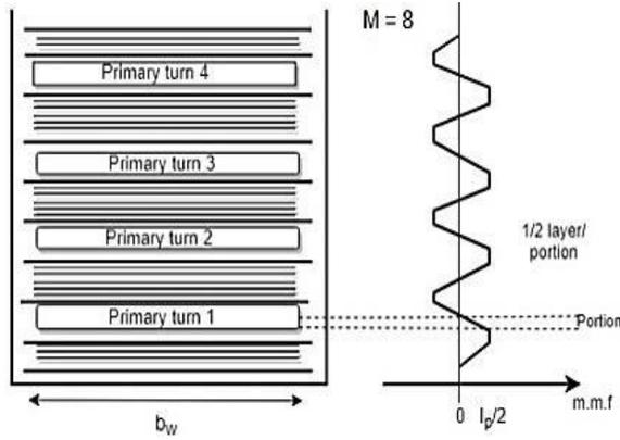
**Fig. 7** Proposed quadruple interleaving transformer winding technique
