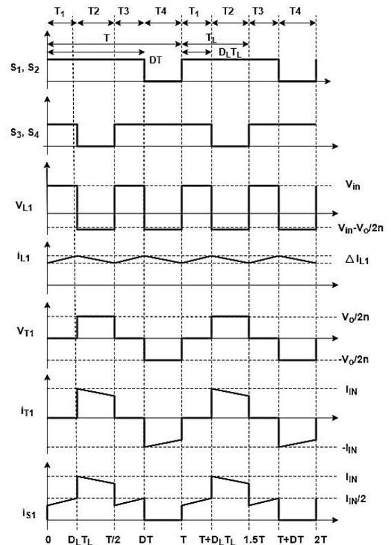
Fig. 3 Operating waveforms of the chosen converter
