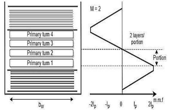
Fig. 5 Conventional single interleaving transformer winding technique
