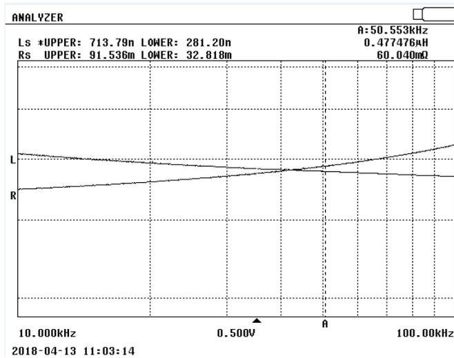
**Fig. 8** Measured ac resistance (R) and leakage inductance (L)
