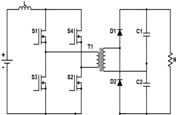
Fig. 1 Full bride isolated boost converter
