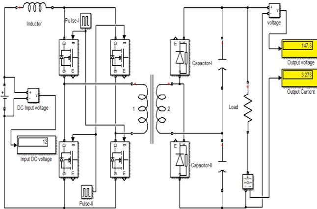
Fig. 2(a) Simulink simulation schematic
