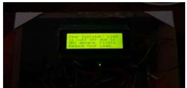
Fig. 4 Load is cut-off due to maximum demand
