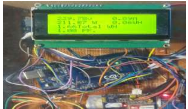
Fig. 3 Parameters measured by Smart Energy Meter
