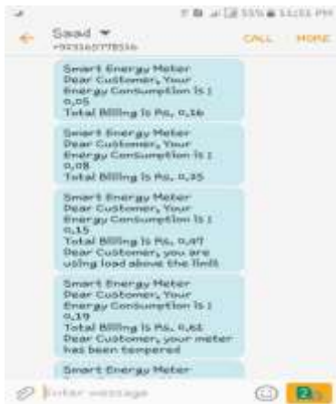
Fig. 7 Smart Energy Meter readings received via SMS
