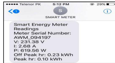
Fig.8. SMS sent by Smart Energy Meter
